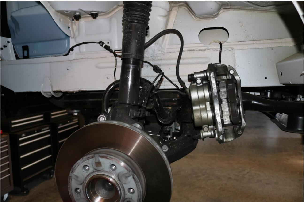
21) Raise the lower control arm about 3/8" (10mm) to remove tension from the strut. Use a 21mm socket to remove the 2 bolts securing the strut to the steering knuckle.
