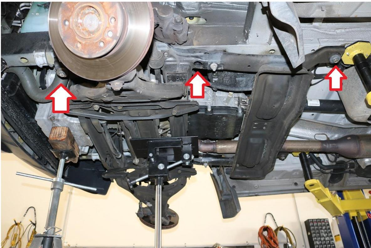
38) Prepare the spacers and new sub frame attachment bolts. The image below shows where each bolt / spacer is designed to be installed. It is critical to use the correct bolts / spacers in their corresponding locations.
