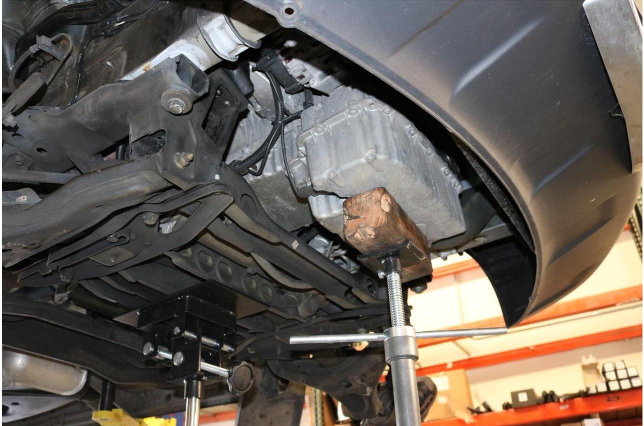
32) Remove the motor mount bolt on both the driver and passenger side with a 16mm socket / wrench.
