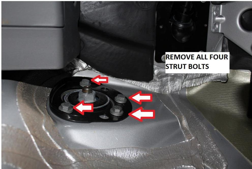
24) The passenger side upper strut bolts can be accessed by pulling up the tool kit cover panel in the passenger footwell. Use a large flat blade screwdriver to rotate the lock knobs on the kick panel so they are horizontal.
