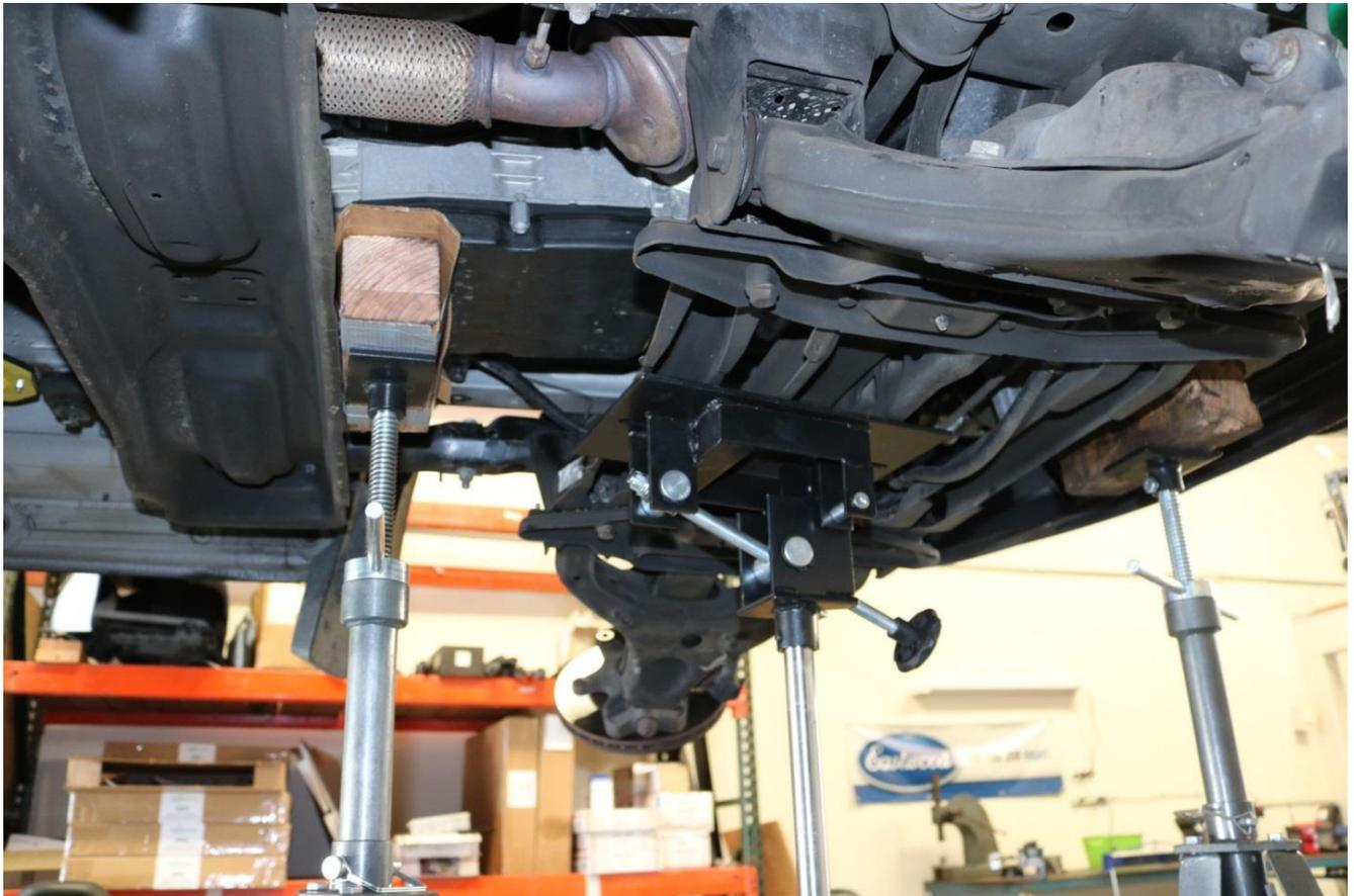
35) Remove the two transmission mount bolts shown below. Use a 16mm socket for removal.
