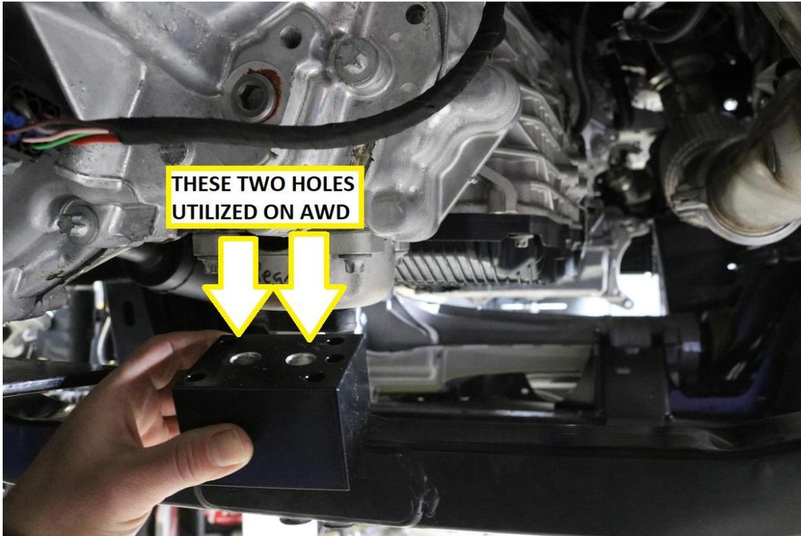
44) Line up the center M10 mounting holes and fit the new M10-1.50 x 130mm long bolts provided. Use a washer under the bolt heads and start the hardware with a 17mm socket / wrench. Do not fully tighten at this time.
