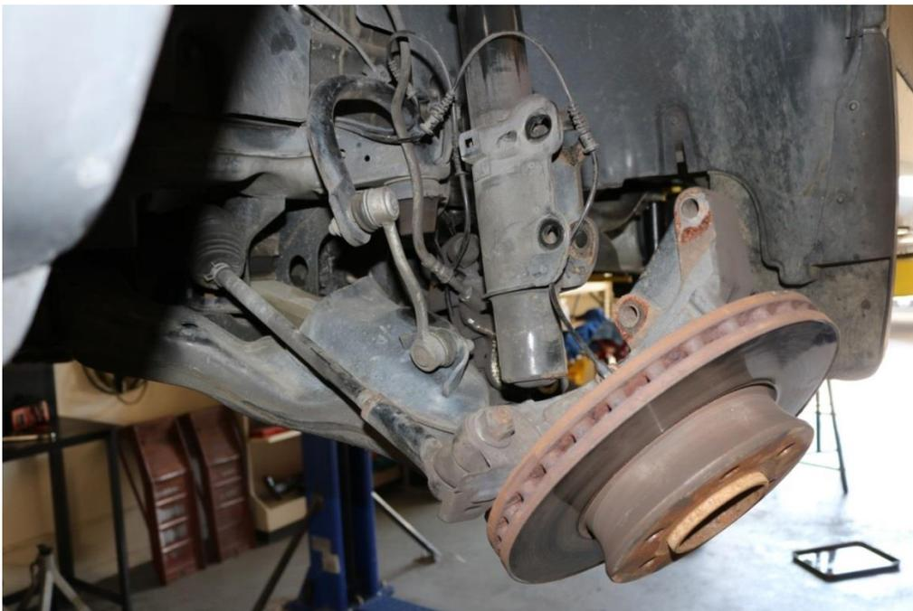
23) Fully remove the strut by removing the four upper strut bolts inside the cabin of the vehicle. Use a 13mm socket / wrench for removal.
