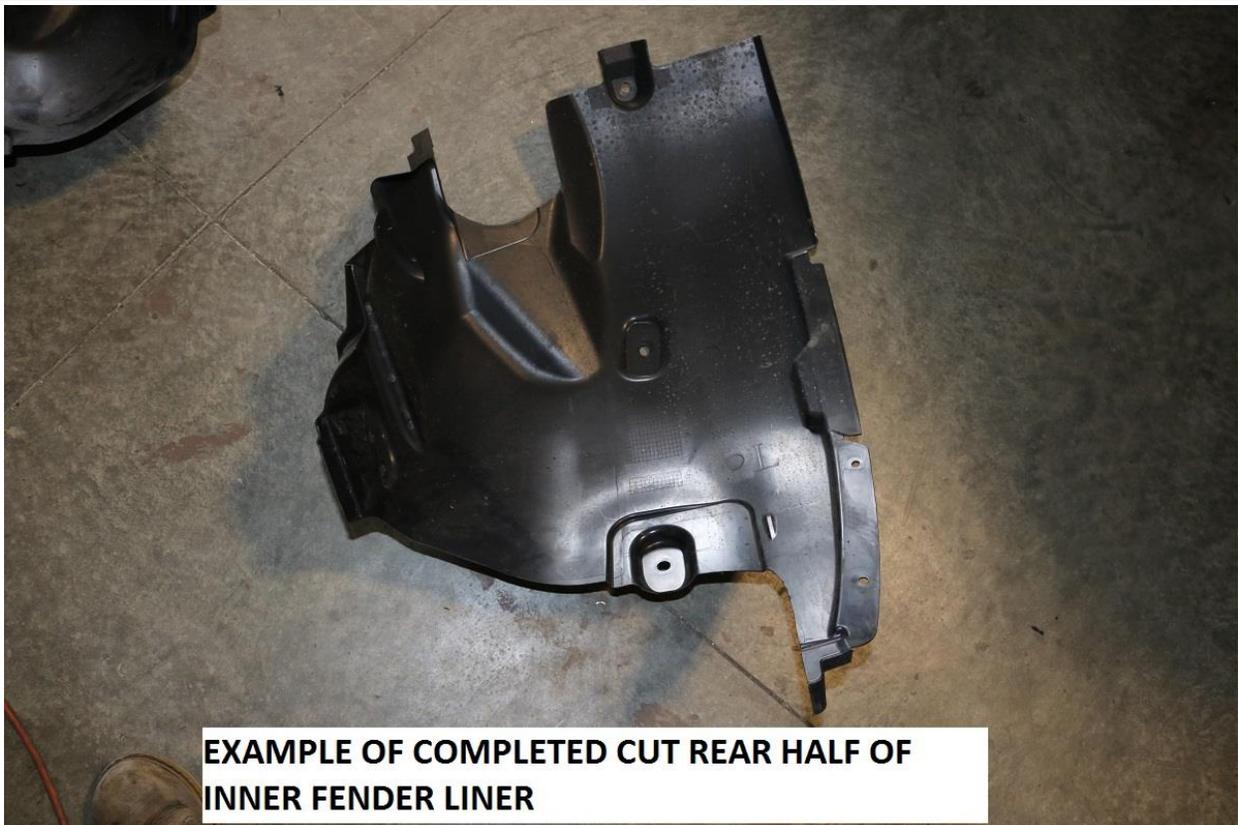
105) Install trimmed fender liners and mudflap as shown below.
