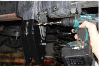
**NOTE:** This Step is MUCH easier if the following are removed: rear coils (not necessary), rearmost exhaust section and rear bump stops. To remove your factory exhaust, pry the rearmost exhaust hanger out of the rubber support and loosen the 15mm factory bolt that clamps the exhaust. If you muscle it, you can break the junction free and remove it; we just spun it out of the way as pictured.
