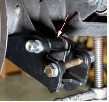
42. Locate the tube crossmember exit on both sides of the frame in front of the rear axle.
