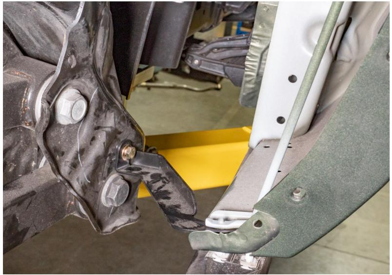
65. Remove the bolt securing the factory e-brake lines to the driver's side rear control arms. Remove the brackets from the crimped sleeves; they will not be reused. We use vice grips and a small pry bar to pry open the clamped area and discard.
