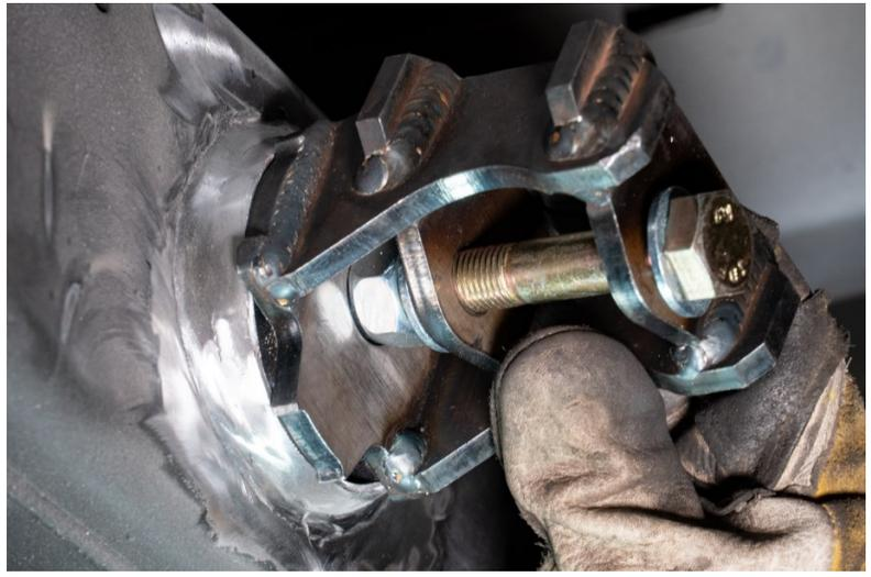
49. Jack the rear axle up until the Carli bump stop drops are resting the bolt heads on the axle strike plates. The passenger's side might hang up a touch (1/8" or so before it hits the bolt heads) as the control arm bolt-heads contact the frame - this is of no concern as the axle will never get there with the bumps installed.
