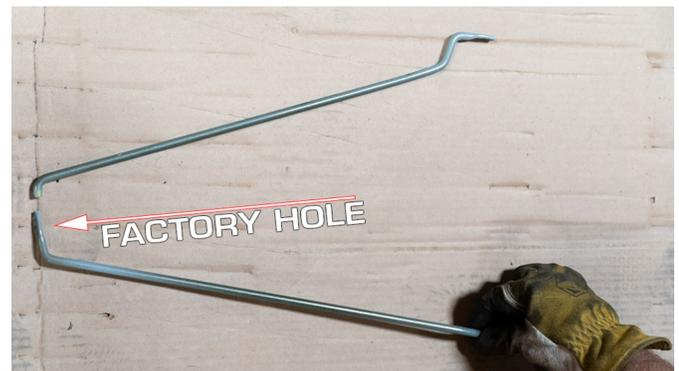
62. Loosely install the Carli bed support to the factory hole above the rear, lower control arm bolt with the provided 3/8"-16 x 1.00" bolt, washers and nut—hand tight for now.
