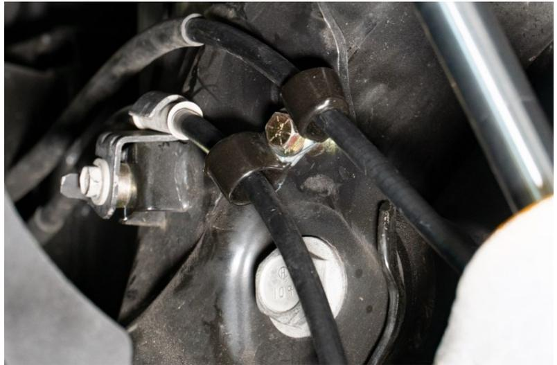
68. On the passenger side, the e-brake cable will likely be touching the back side of the shock; use vice grips to bend the factory routing bracket on the inner side of the passenger control arm mount upward to ensure the brake lines clear the shocks at full extension.
