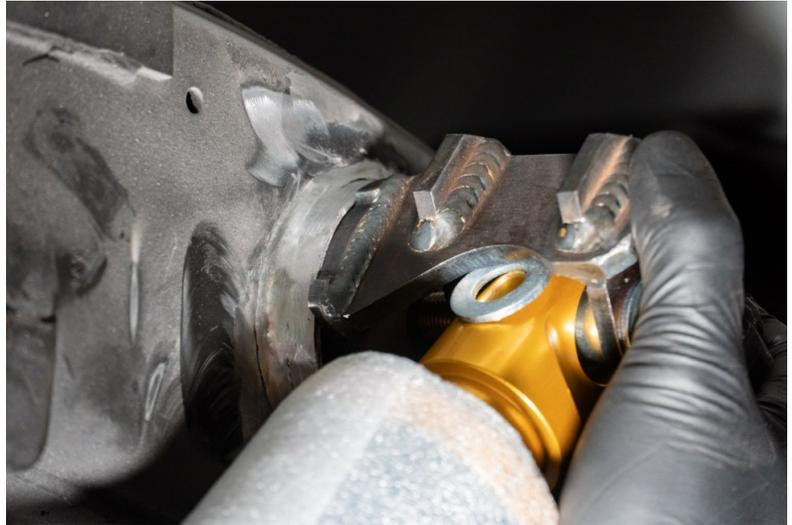
54. With the tack welds in place, remove the spacer and inspect everything. The rear end should be completely bottomed out with the rear track bar drop installed (Track bar pivot bolts loose), the rear shock installed loosely into the mounts, upper mount tack welded in with only a small gap between the rod end and shock mount (plenty of room for shock to swing down).
