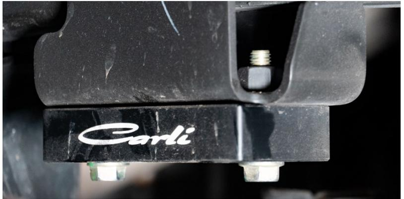
37. Install the Carli Lower Shock Mount. The mount itself will slide over the factory lower shock mount. Remove all hardware and slide the Carli shock mount over the factory mount from front to back, not bottom up.
