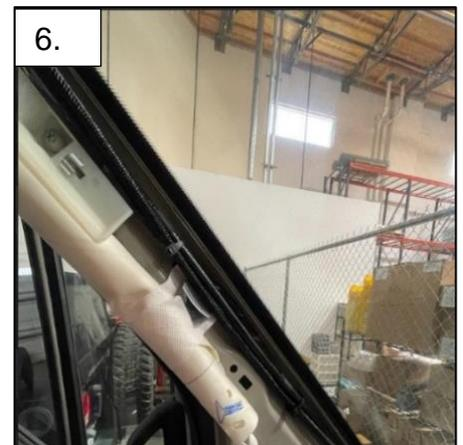
7. Using a T27 screwdriver, remove the two bolts holding the sun visor in. There is one on the right and left. The right one will be exposed with the sun visor closed, and the left one will be exposed with the sun visor open. Remove the sun visor.
