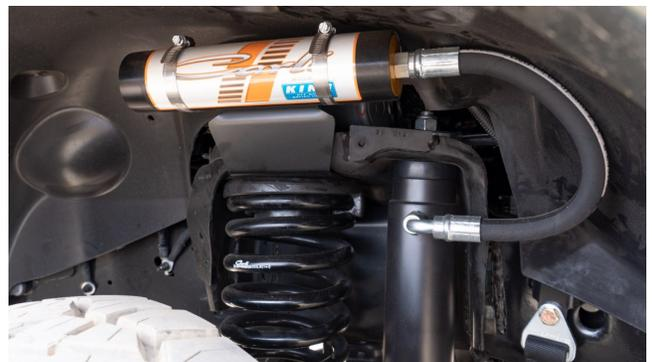
10. **Torque the lower shock bolt to 100lb.ft. (125lb/ft. if running Carli Lower Shock Mounts)**
