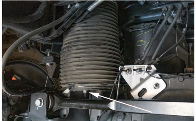
24. Remove the factory position sensor links from the armature and axle mount. These will pop off with force—be careful to not damage the sensor arm.
