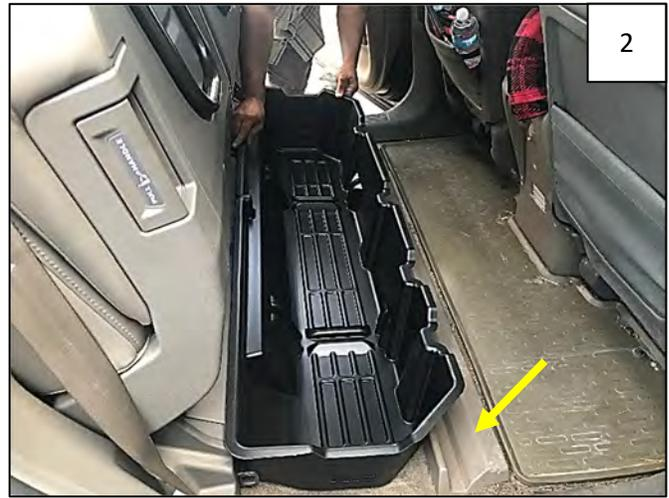
Nest the Underseat Storage Box behind molded seat support feature on floor (indicated by arrow).
