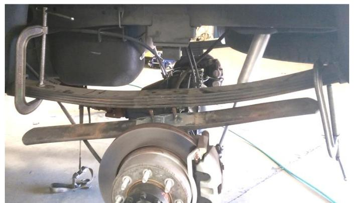
10. Remove the Bolt, sleeve and nut from the spring retainer clamps and temporary center pins from the add-a-packs.
