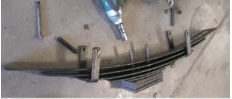
12. Install add-a-pack to the bottom of the leaf spring pack ensuring the center-pin holes are properly aligned. Use a C-Clamp to cinch the pack together and thread the nuts on hand tight.
