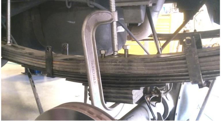
14. Tighten the nuts until the pack is cinched together fully, then remove C-Clamps.
