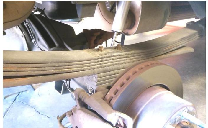
7. Secure spring assembly together with 2 C-clamps on outer edges of lower leaf. Do not include the thick, overload leaf on the very bottom.
