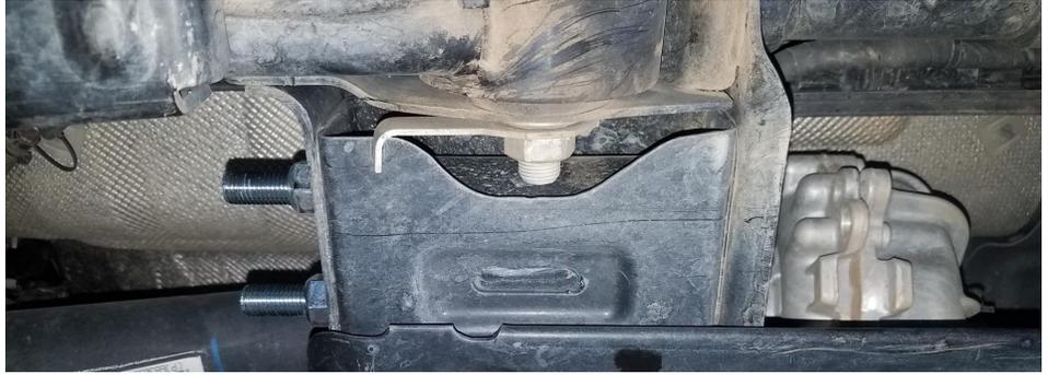
3. On the passenger's side, the Catalytic Converter impedes removal of the factory bolt. Leave the factory nut engaged a couple threads and push the bolt-head away from the crossmember.
