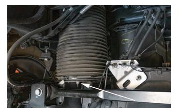
24. Remove the factory position sensor links from the armature and axle mount. These will pop off with force—be careful to not damage the sensor arm.
