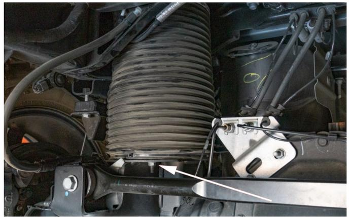
22. Remove the factory position sensor links from the armature and axle mount. These will pop off with force—be careful to not damage the sensor arm.
