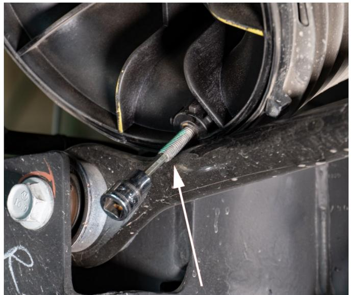
25. Install the Top half of the Carli Airbag spacer to the bottom of the air-bag using the provided M8x16mm Button head bolts. **SNUG** These, do not overtighten as they’re going into a metal sleeve in a plastic bag piston. **DO NOT USE AN IMPACT.** **NOTE:** There are two pins installed in the Carli upper brackets; this marks the REAR; these will sit tight to the back of the lower bag piston as a failsafe.
