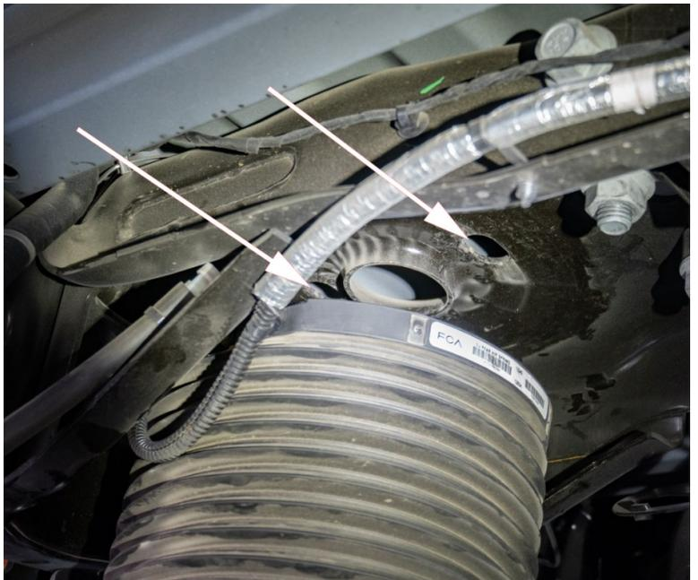
35. Use a 15mm socket to remove the factory bump stops from the frame rail—Install the Carli bump drop with the Provided Extended M10 hardware between the frame and factory bump stop.
