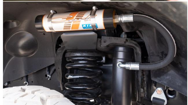
7. **Torque the lower shock bolt to 100lb.ft. (125lb/ft. if running Carli Lower Shock Mounts)**
