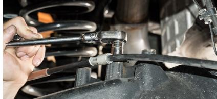
13mm Socket - Remove the bolt securing the brake line bracket to the inside of the passenger's side control arm bracket.
