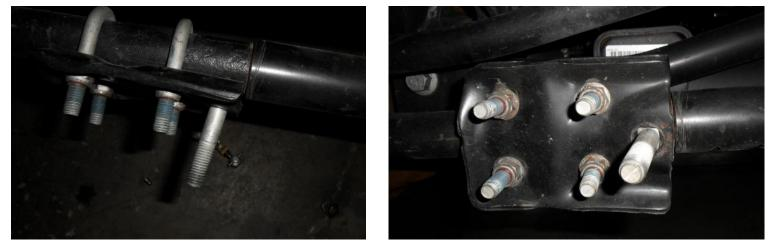
5. Tighten the U-bolts on factory stabilizer clamp to 45 lbs/ft and make sure the bracket is facing straight out. Install the 2 gold spacers from the Hardware kit onto the stud, then place the Body end of the shock onto the stud, one more gold spacer, then install factory nut. Tighten nut to 30 lbs/ft.
