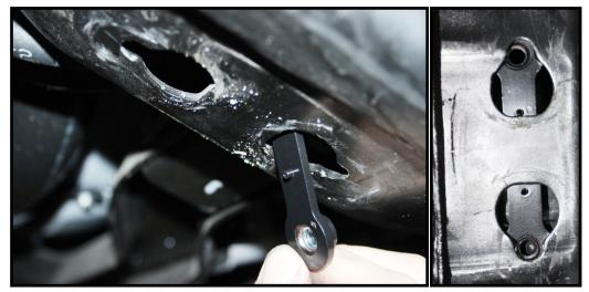
6. Insert the provided captured-nut bracket into the frame rail. The insert indexes into the opening - it should sit flush against the inside of the frame rail with the threaded inserts facing upward into the frame. The indexes will rest against the center-portion of frame between the openings.
