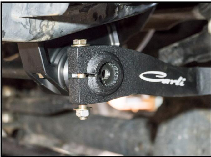
12. With both sides installed hand tight, torque the 3/8-16 x 2.5"bolts to 5lb.ft.
