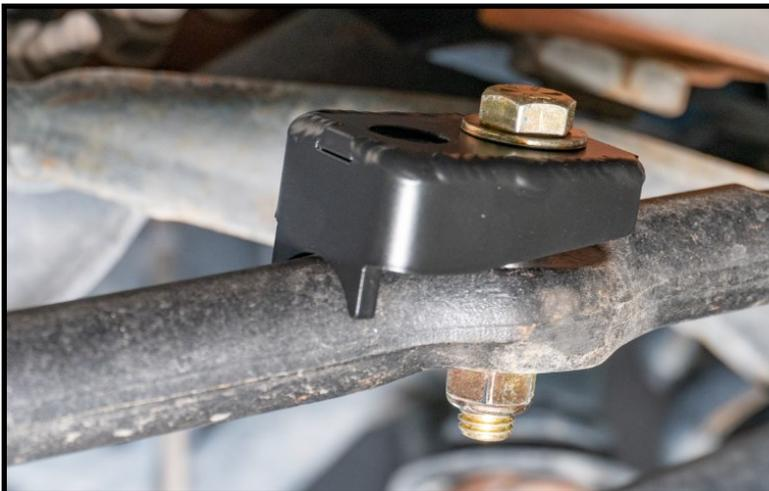
10. Coat the threads of the stainless stud with blue Loctite and thread into the welded nut in the installed drag-link Clamp..
