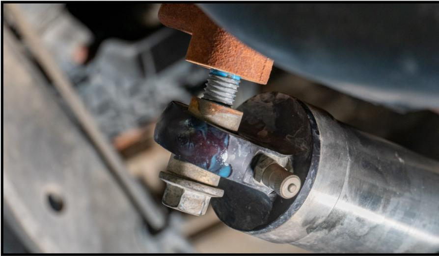
12. Coat the threads of the factor bolts with blue Loctite and slide one bearing spacer over the shank.
