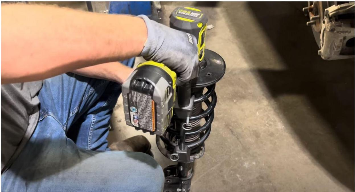
7.Remove the black metal top of the strut and then the green plastic spring seat underneath.
