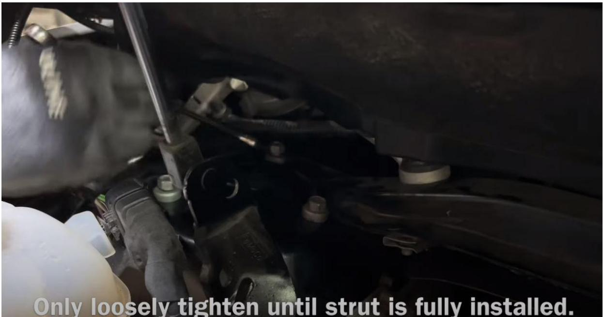
13. Reinstall the mounting bolts, sway bar link, brake line bracketry and tighten fully.
