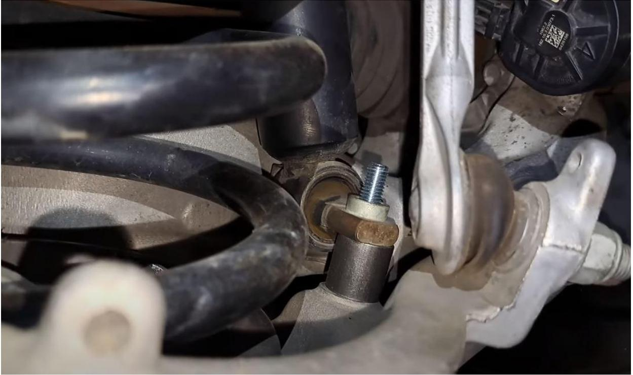
22. Reinstall the nuts and bolts on rear suspension lower control arm.
