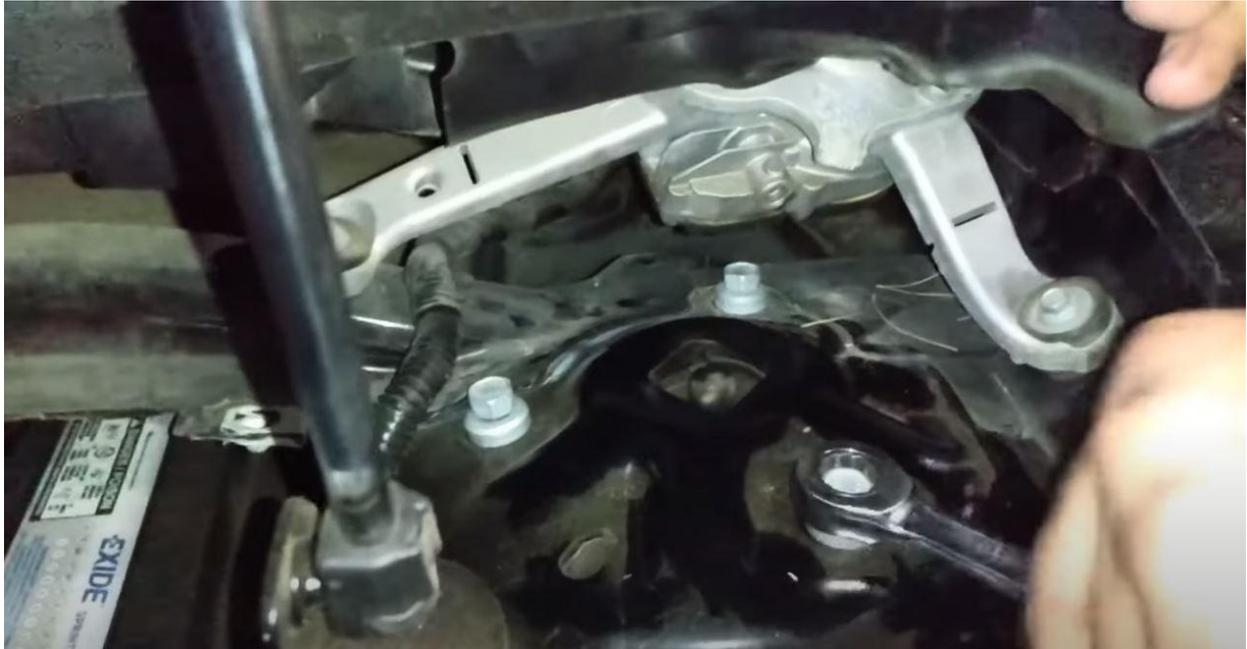
4. Remove the rest of the mounting bolts/brake line bracket/sway bar link from the lower strut area.
