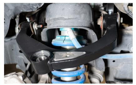
11. Lightly coat the upper misalignment spacer and lower knuckle pin with grease and insert them into the uniball. These are a very tight fit and may require a light tap with a rubber mallet to drive in.
