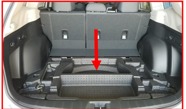
Locate the plastic push clips holding the foam tool holders in place. Remove these clips and set the foam pieces aside.
