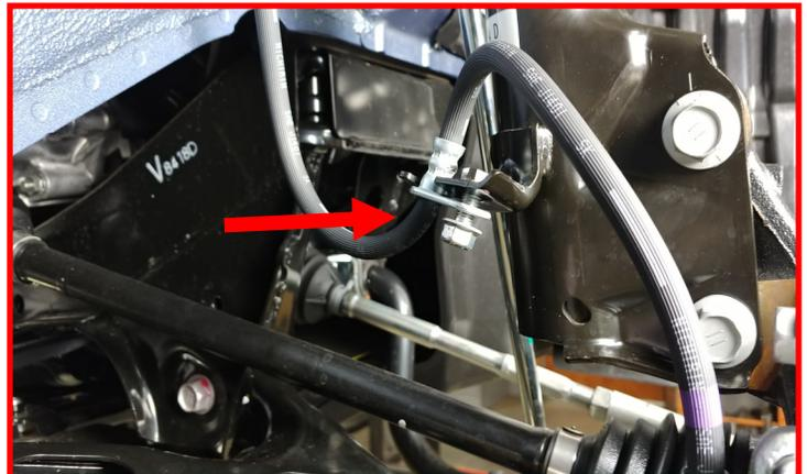
Remove the ABS harness clip at the strut body. Let hang out of the way.
