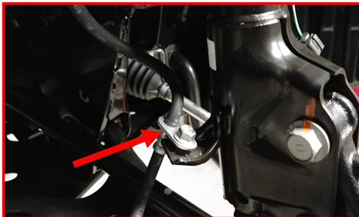
Remove the factory end link from the sway bar. Remove from vehicle and discard.
