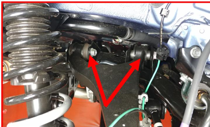
Loosen but do not remove the front lower control arm bolts.
