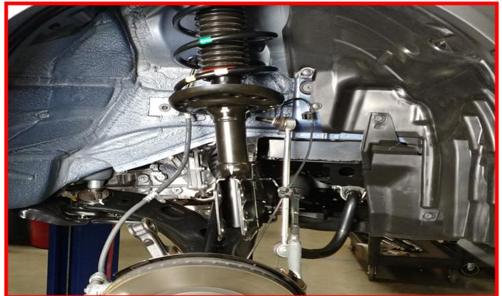
Raise the knuckle up and install into the strut body. Install the cam bolt into the upper hole and the remaining bolt into the lower.
