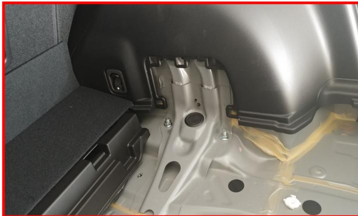
Remove the strut nuts and set aside.
