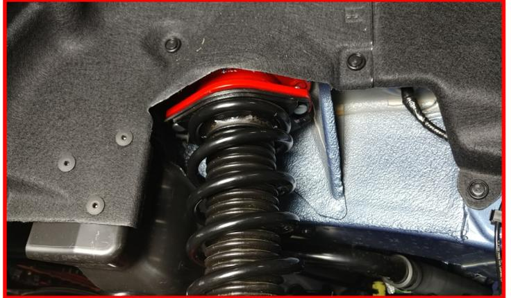
Raise the lower control arm into place and install the **lower strut hardware**. Do not tighten at this time. Use the jack and raise the lower control up to set pre load on the strut. Install the lower **knuckle bolt**. Do not tighten at this time.
