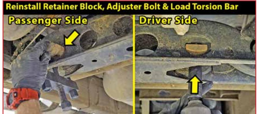
Load the torsion bars. Reinstall the retainer block and bolt. Run the adjuster bolt 'all the way' up to fully load the torsion bar. {22mm} (It's easier to 'unload' the torsion bars to adjust the height, than it is to add load.) This adjustment will be changed at the end of the installation.
