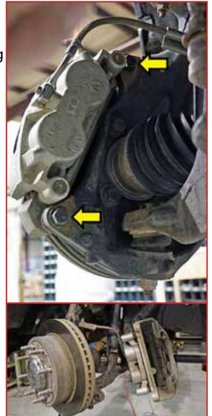
**REMOVE HUB DUST COVER & ROTOR...**
