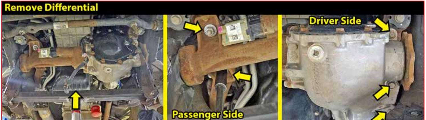
[Illustration 23B] **TECH TIP:** The top rear bolt is hard to reach. You may have to access the bolt from the rear by going through the opening near the driveshaft. Our tool of choice was a small ratchet with a swivel socket, a 3 inch extension and 15mm socket.
