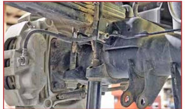
Make sure the locating pins are seated correctly. Jack the axle back into position while making sure that the axle pins are seated correctly into the block.
