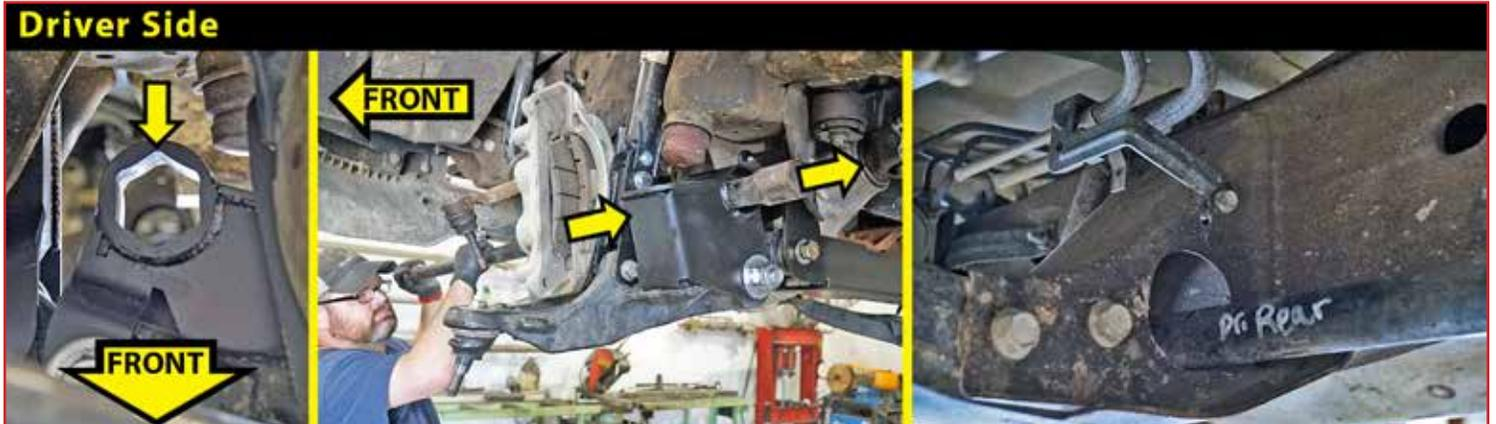
[Illustration 42B] Locate the torsion bar adjuster arm/torsion key. Slide the torsion key up into the crossmember. Slide the torsion bar into the hex opening and completely through the key. The torsion bar should be locked into position in the front SUPERLIFT torsion bar bracket.
