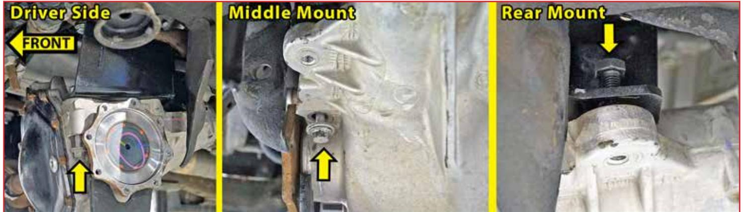
□ 29. [Illustration 29] Fasten the Passenger side with the provided (2) 12mm-1.75 x 40mm Bolts, (2) 12mm Flat Washers and (2) 12mm Stover Nuts - Bolts Pointing Down. Apply thread locking compound to the threads before installation. {19mm} (74).
