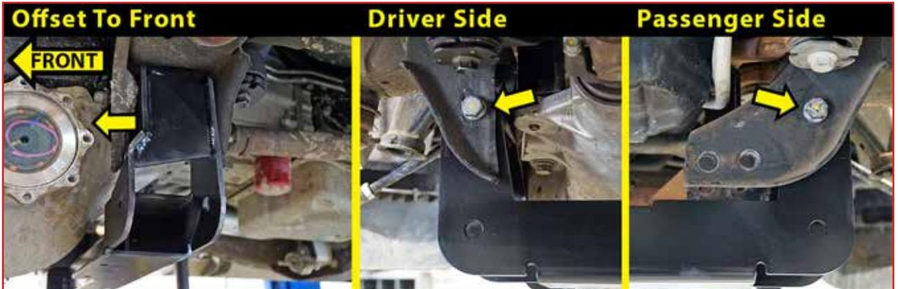
□□ 33. [Illustration 33] Locate the SUPERLIFT front crossmember (#55-05-3350). **NOTE:** The offset bend goes toward the 'Front' of the vehicle. Hang the Driver side, then swing the crossmember to install the Passenger side.
