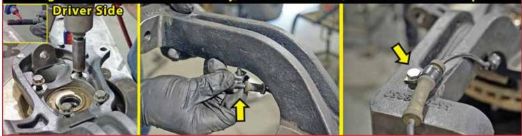
**STEERING KNUCKLE INSTALL...** []] 47. [Illustration 47] Position a jack or jack stand under the knuckle assembly. The assembly is heavy and you may need to lift or lower to install the knuckle.
