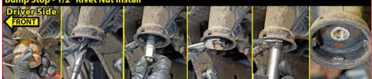
35. [Illustration 35] From the inside looking out, locate the factory hole just above the bump stop cup. Using the factory hole as a guide, use an 11/16" drill bit to enlarge the hole for the 1/2" rivet nut.
