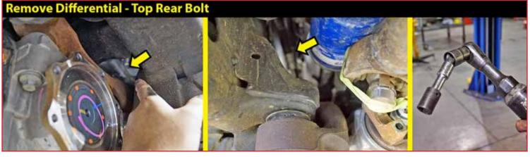
24. [Illustration 24] Disconnect the axle breather tube from the top of the Driver side of the differential.
