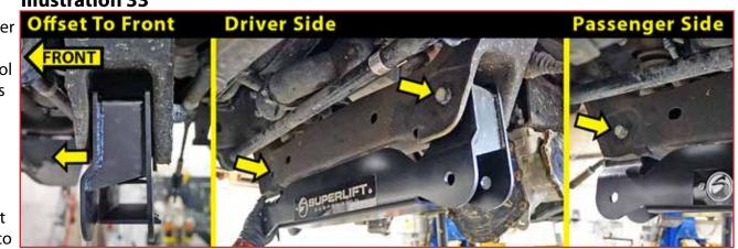
Rear. {21mm wrench / 24mm socket} Leave hardware loose.
