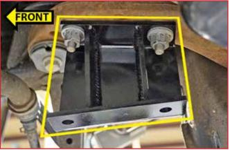
27. [Illustration 27] Locate the SUPERLIFT Driver side differential bracket (#55-03-3350). The Bracket has a open side that goes toward the 'inside' of the vehicle (the flat side goes toward the 'outside.)
