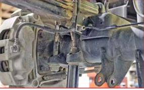
Make sure the locating pins are seated correctly. Jack the axle back into position while making sure that the axle pins are seated correctly into the block.
