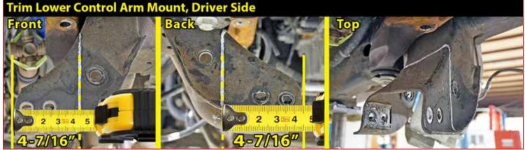
**CAUTION:** When using a torch or plasma cutter, beware of the sticky, waxy undercoating - cosmoline. This will melt and drip during the cutting process. Take precautions to cover your person and the floor from this extremely HOT material.
