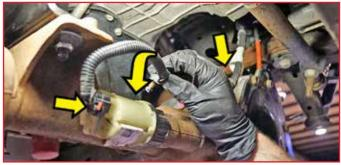
31. [Illustration 31] Locate the front driveshaft factory clamps/bolts. Apply thread locking compound to the factory clamps/bolts threads before installation. Alignment mark on the front driveshaft and front differential input voke, reconnect the front driveshaft to the front differential. {11mm} (25)
