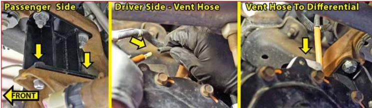
□ 30. [Illustration 30] Connect the electrical connector from the front differential actuator.
