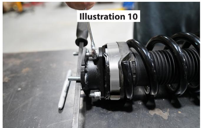
26. Attach the strut spacer assembly onto the top of the strut by aligning the strut spacer assembly onto the three (3) factory studs. Secure using the factory hardware. [15mm] (40)
