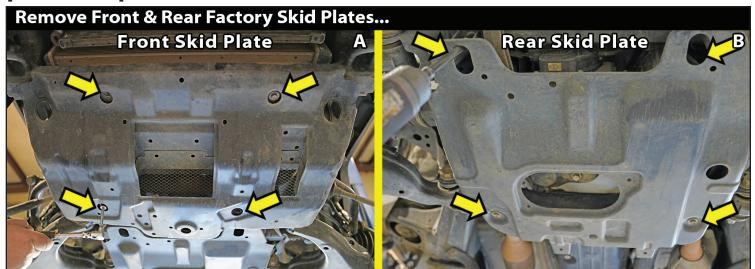
TECH TIP When you remove a factory nut or bolt, like the skid plate fasteners, sway bar links, ball joint nut, etc., put it back into the factory spot for safe keeping. You will not have to look or sort through removed hardware to find the proper factory fastener.
