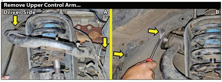
[Illustration 8-C & 8-B] Push the upper control arm bolt toward the front of the vehicle until it contacts the body. Mark where bolt contacts body. Push bolt back into control arm. Using pliers or an adjustable crescent wrench, slowly bend body out at mark to provide clearance to remove the upper control arm bolt.
