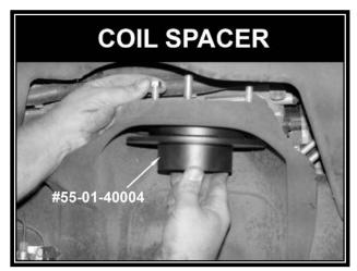
**NOTE:** On some models the driveshaft must be disconnected at the axle to allow the axle to drop sufficiently for coil / spacer installation.
