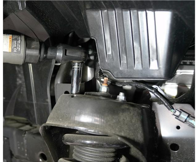
10. Install the strut spacer onto the strut and secure using the factory hardware. [14mm]
