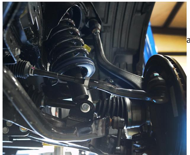
6. If equipped, unclip the two lines from the upper control arm, remove the upper control arm bolts then remove the arm from the truck. [19mm]
