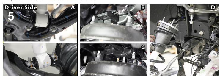
21. [Illustration 6] With the lower control arm still supported with a jack, remove the upper control bolts and remove the upper control arm from the vehicle. [21mm]
