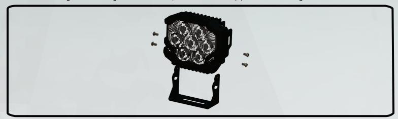
3. When reinstalling the M6 screws, do not use a power tool and do not overtighten!
