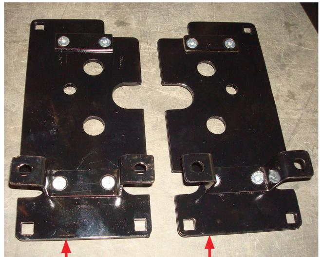
Left (driver's) side frame bracket assembly      Right (passenger's) side frame bracket assembly      Fig. 10
