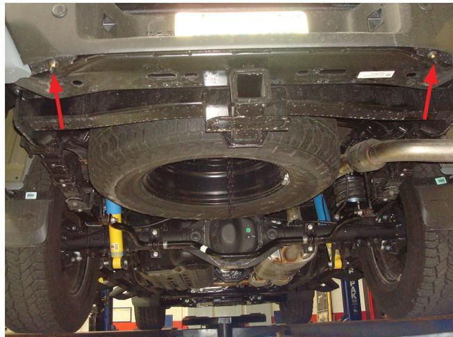
Back view showing valve locations and air spring assembly installed.
