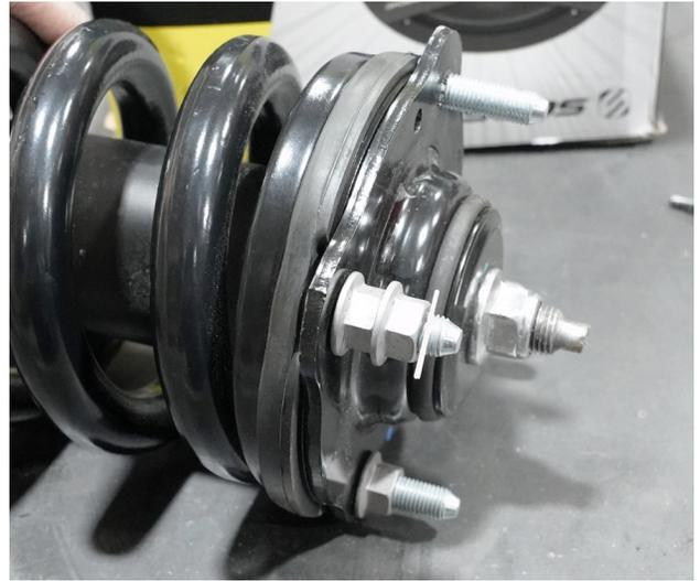
11. All the factory studs need to be trimmed before installing the strut spacer, mark each stud by threading on two of the supplied 10mm flange nuts and marking the stud at the top of the second nut.
