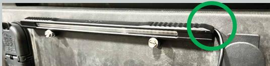
2. Drill a 1/4" hole in your bumper and pass the wiring through. and reinstall your license plate with Boost Bar.
