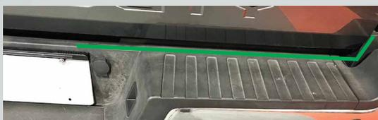
4. Run the wiring up through the tail light hole and plug into your RIGHT Morimoto tail light. Secure remaining wiring with zip ties.
