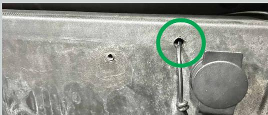
3. Run the wiring behind the bumper along the top, and secure using zip ties.
