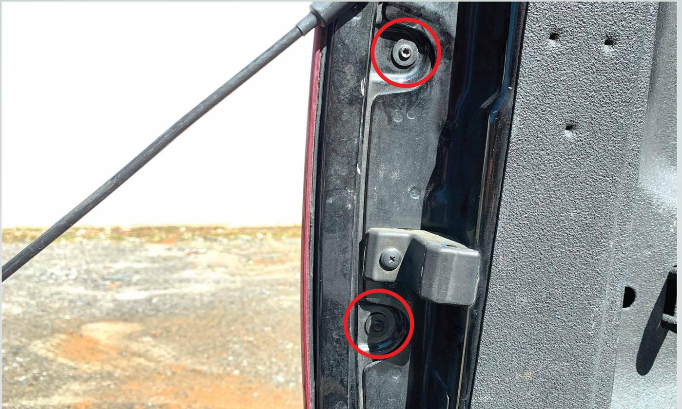
2. Insert a plastic trim tool in the gap shown below and pry the tail light backwards away from the bed.
