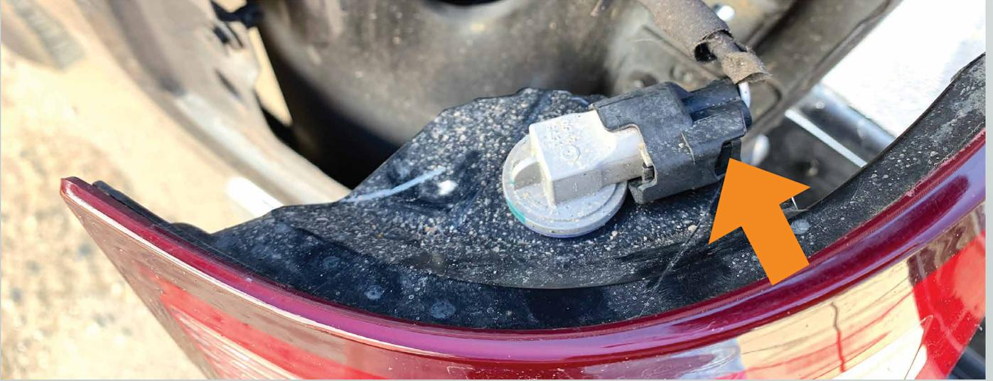
5. Grab one Morimoto tail light of the same side, locate the included incandecent adapter and plug it into the Morimoto tail light (#1). The other side of the adapter plugs into the OEM harness (#2).
