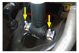
11. Remove the mounting nut holding the anti-sway bar end link to the lower control arm. The nut is located on the underside of the lower control arm. This will allow the lower control arm to swing down and ease the removal of the strut.
