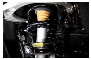
26. Attach the lower strut mount to the lower control arm with the two OEM bolts and torque to 37 ft lbs.
