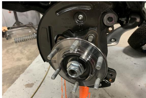
17. Break loose but do not remove the upper and lower ball joint 18mm nuts. Use a ball joint separator tool to detach the ball joints from the spindle. Alternatively with a hammer, you can strike the ball joint boss on the spindle to remove the ball joint.
