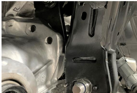
40. Tighten and torque all differential bolts to OE specs. Reconnect all electrical connections and hoses.
