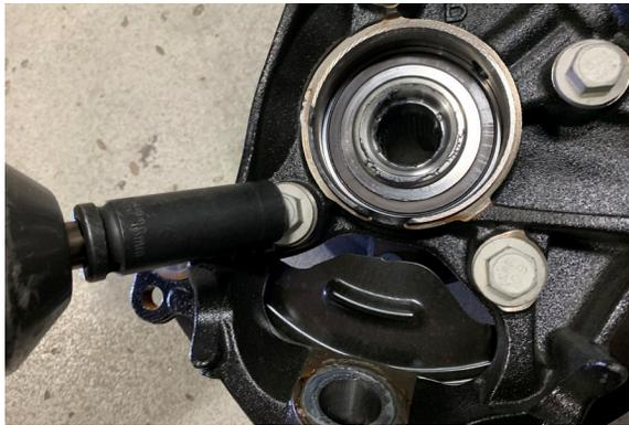
20. Remove the three 15mm top mount nuts holding the strut to the chassis and the two lower strut 18mm nuts. Lower the control arm assembly to gain clearance for the strut to be removed from the vehicle.
