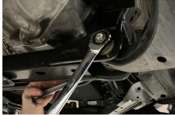
23. Disconnect all hoses and connectors from the front differential. This will prevent damage or over stretching to any hoses, lines, or cables. (This step will vary depending on the vehicles equipped options.)
