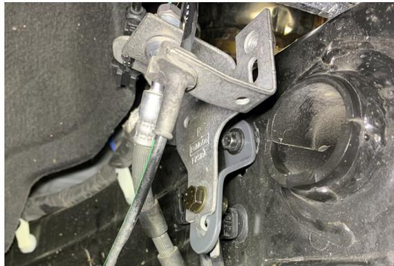
46. Attach the wheel speed sensor to the spindle and torque to 71 *in lb*.
