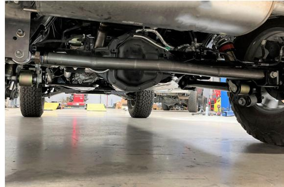
67. Detach the brake line bracket from the top of the axle on the passenger side.
