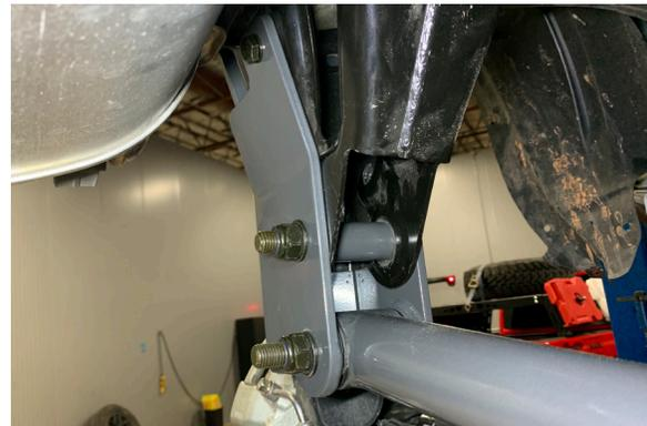
62. Insert the two supplied M12 bolts with nuts and washers through the front and back holes near the base of the bracket.
