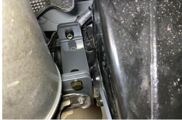
64. Attach the original exhaust hanger bracket to the chassis with the original hardware.
