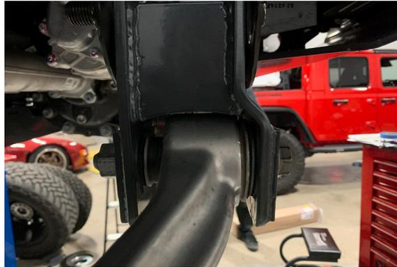
44. Install the new assembled Belltech spindle onto the upper and lower ball joints using the original nuts. Torque the lower ball joint nut to 85 ft lbs. and the upper ball joint nut to 46 ft lbs. Ensure to reattach the brake backing plate that was previously removed.
