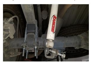
31. Loosen the 21mm U-bolt nuts evenly until removed. Detach the original U-bolts to remove the factory blocks. Slowly lower the axle using the jack to install the new Belltech lift blocks.
