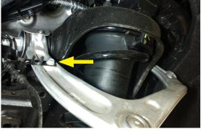
12. Use a 18mm and 9mm wrench to disconnect the sway bar from the end links.
