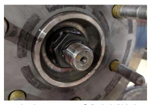
15. Break loose the upper ball joint 18mm nut but do not remove yet. Strike the ball joint boss with a dead blow hammer to dislodge the upper control arm from the spindle. Allow the spindle to droop as you slide the axle shaft out of the hub.
