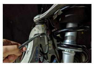
16. The struts must be removed.
