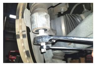
10. Place a jack underneath the lower control arm to support the assembly and loosen the top and bottom control arm bolts to allow the control arms to move easier.
