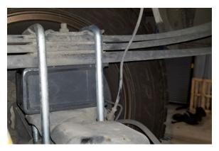
33. Use the jack to apply slight pressure at the rear axle to keep the pin aligned. Install the supplied Belltech U-bolts and tighten in a crossing pattern; then torque to First Pass: 59 ft lbs., Second Pass: Loosen 180 degrees, Third Pass: 59 ft lbs., Final Pass: 120-140 degrees.
