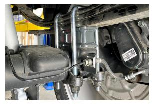
34. Mount the new Belltech shock absorbers using the original hardware. Torque the upper bolt to 70 ft lbs. and the lower nut to 118 ft lbs.
