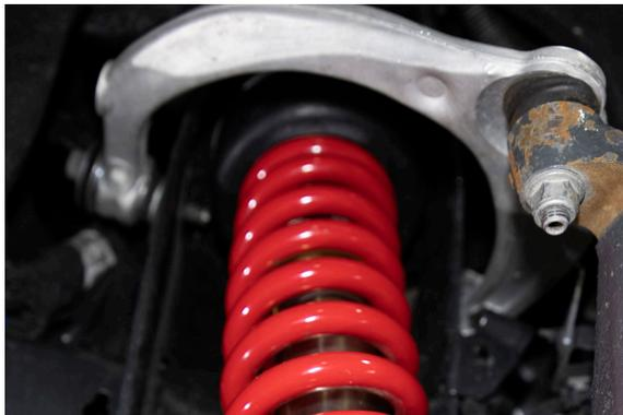
27. Attach the lower strut mount to the lower control arm using the supplied bolts, washers and Nyloc nuts. Torque the supplied nuts to 60 ft lbs.
