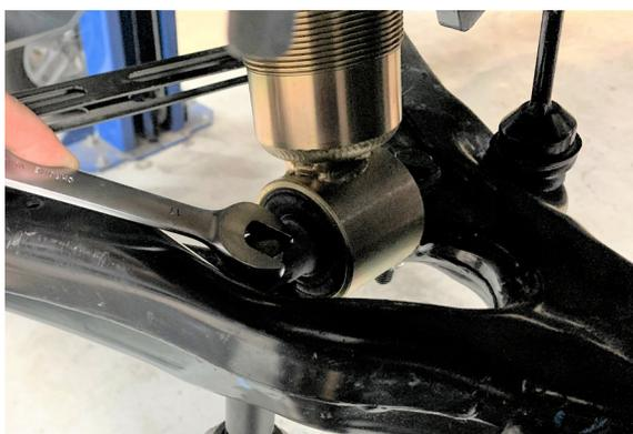
28. Attach the end link to the lower control arm, torque to 74 ft lbs. when the suspension is loaded or the vehicle is back on the ground.
