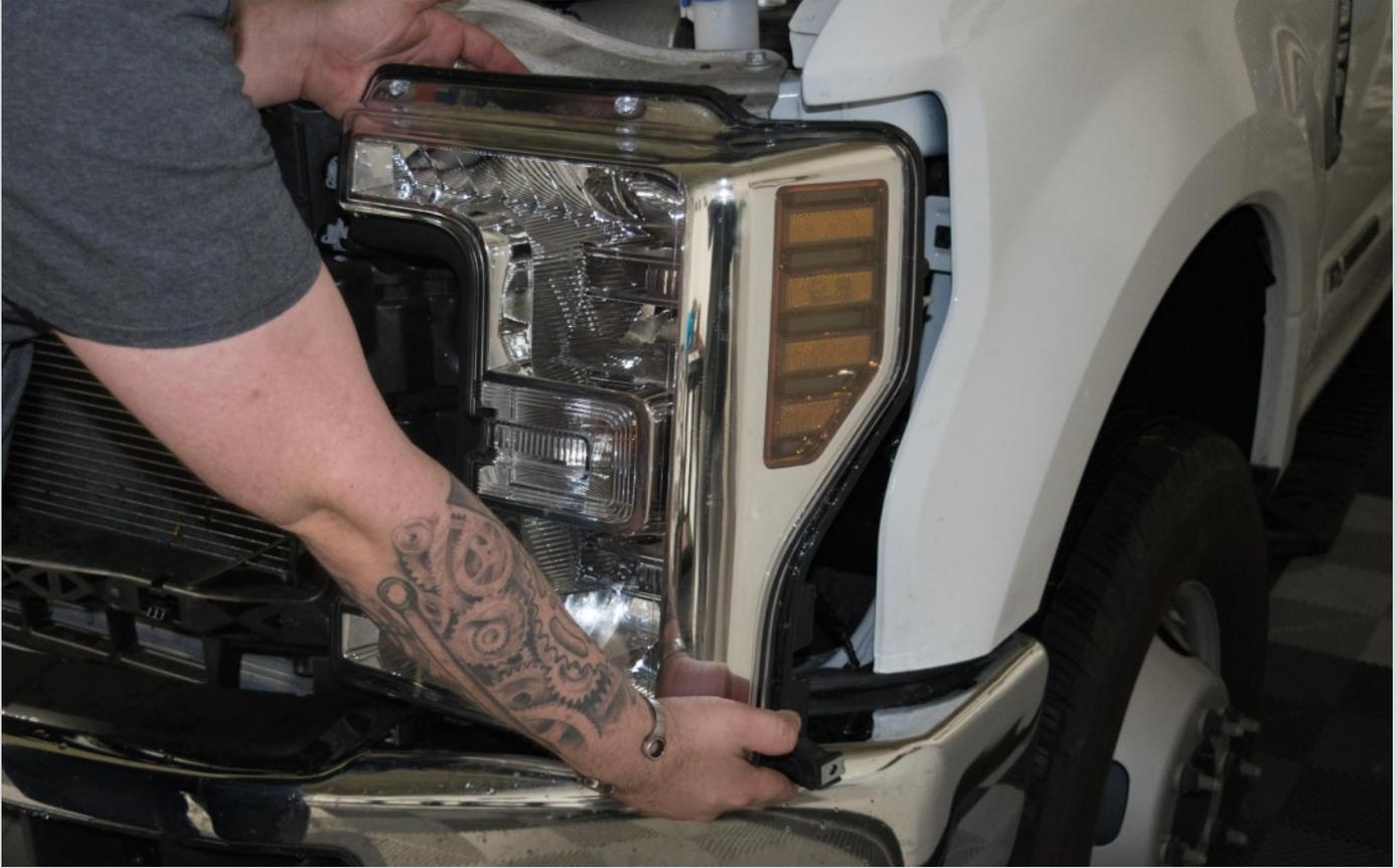
8. Unplug and remove each electrical connection from the back of the housings. For the halogen trucks, there are four electrical plugs to remove from the back of each housing.
