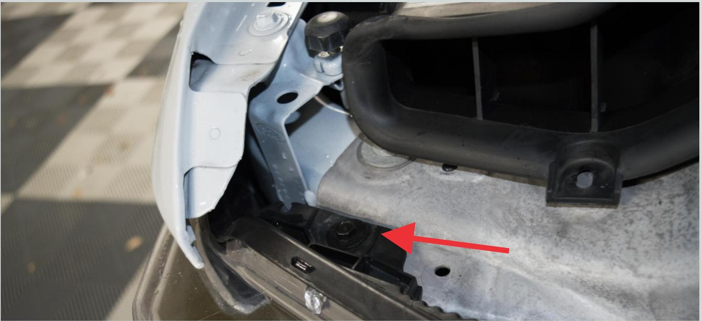
6B. The most difficult bolt to access is indicated. It is best removed with patience and a ratcheting 10mm closed-end wrench and is accessed via a very slim opening between the fender liner and bumper. There is one of these bolts per headlight (two total).
