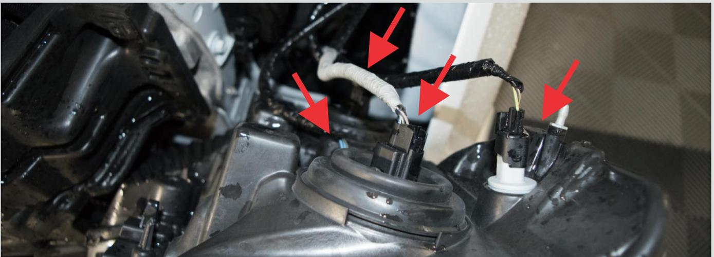
9. Connect stock headlight connectors to the Morimoto headlights. Refer to page 2 or 3 for identification. There are two H13 connectors per headlight. Use the H13 connector with the black wiring loom and not the grey loom as indicated.
