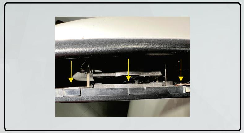
3. Tilt the mirror glass down then pull it up to separate it from the assembly.
