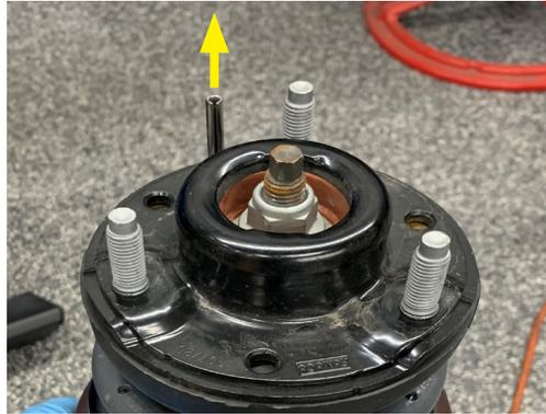
35. Place the top mount studs through the upper strut spacer and fasten the spacer on the strut using original hardware.
