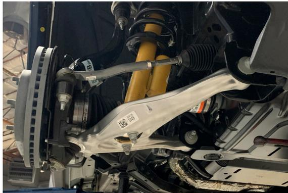
28. Reattach the sway bar end links to the lower control arm, torque to 111 ft lbs.
