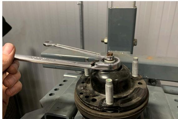
17. Detach the upper spring isolator from the top mount. If needed, use a pry tool or flathead screwdriver.
