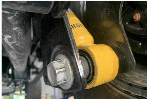
32. Remove the 15mm upper strut mount bolts.
