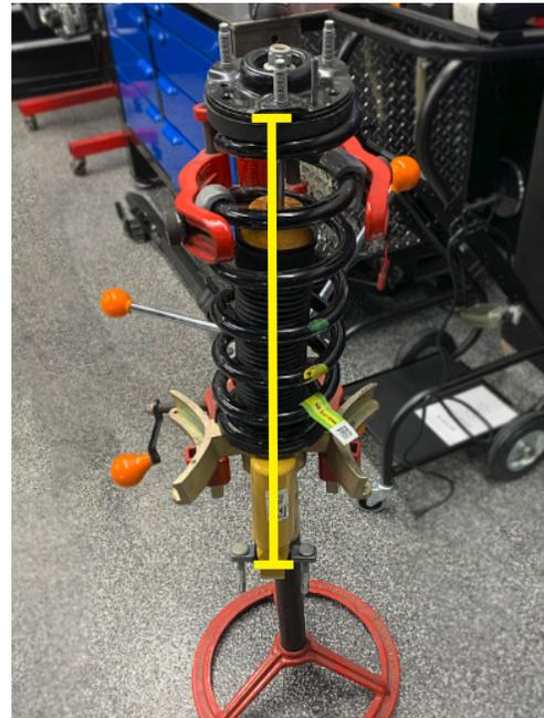
16. Support the strut to prevent it from falling from the fixture as you remove top mount and the strut.
