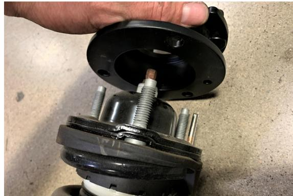
35. Secure the spacer with the split washers and M10x1.5mm nuts. Spin the nuts until snug then tighten using an open ended wrench or thin wall socket.
