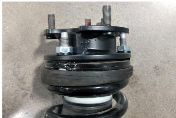
36. Mount the strut and spacer assembly on the vehicle.
