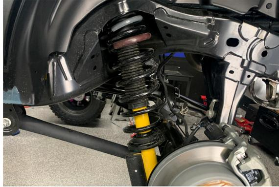
38. Attach the lower strut bolt and nut, torque to 350 ft lbs.
