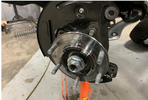
14. With a 15mm wrench, remove the three top mount nuts holding the strut to the chassis. Lower the control arm assembly to gain clearance for the strut to be removed from the vehicle.
