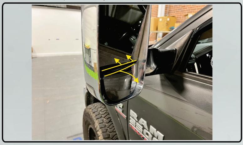
2. Unplug the stock mirror light's connector. Remove the one (1x) T15 screw holding the mirror light in.
