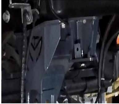
Use the factory bolt to attach the bump stop extension to the frame. Next, use the provided M8-1.25x30mm hardware to attach the bump stop cup to the extension.
