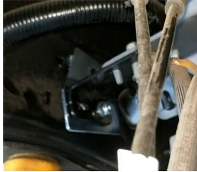
Unbolt the rear brake line bracket that is mounted on the driver side frame. Next, slide the new max-trac bracket in-between the frame and the factory. Use the provided hardware to mount the Maxtrac bracket to the frame and the OE hardware to the connect the OE bracket to the Maxtrac bracket
