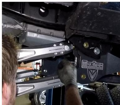
Install the 4 link arms at this time. Start with the upper arm then the lower arm. Use the provided 9/16-12x4 & x 5" bolts for the links at the hangers, Then use the provided M18 X 140 bolts and steel sleeves at the axle to mount the arms. Next, insert the clamp bolts and tighten.
