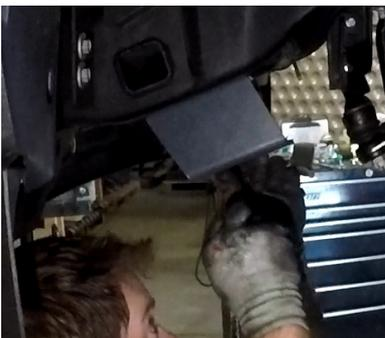
Install the sway bar drops to the OE sway bar mounting studs on the frame using the previously removed OE hardware.
