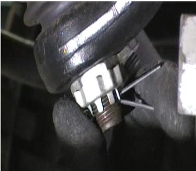
Remove the sector Pitman arm retaining nut and save for re-installation. Use a Pitman arm puller to remove the OE pitman arm. The threads of the sector shaft and the Pitman arm retaining nut must be cleaned of all factory dry adhesive
