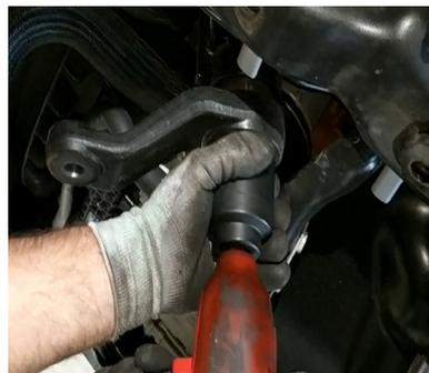
Reinstall the Pitman arm retaining nut to the sector shaft and torque to 350 ft./lbs.
