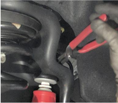
On the driver side, unclip the axle vent line from inside the frame.
