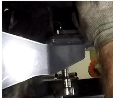
Insert the link arm bracket inside of the original radius arm pocket. The brackets are side specific and will display the Maxtrac logo outwards. While holding the bracket up, line the two holes up and insert the provided M18x130 bolt into the original radius arm bolt hole. Next, install the reduction spacers into the smaller holes just in front of the M18 bolt. Do not install the bolt until the arm is installed
