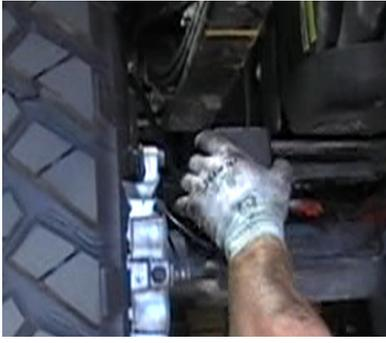
Lower the rear axle and remove the factory block.
