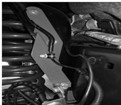
Attach the vacuum lines to the Maxtrac brake line bracket using the provided adel clamps using the 6mm hardware
