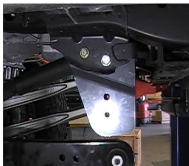
Place a jack under the pinion or radius arm. On both sides remove the rear bolts holding the radius arms to the frame of the vehicle. Carefully rotate both radius arms down to provide adequate space to install the new drop brackets. Install the radius arm drop brackets using the supplied 18mm X 130mm bolts in the front holes with the heads of the bolts facing out. Do not torque at this time.
