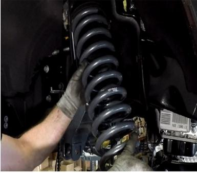
Using the factory isolators install the supplied front coil springs into the spring buckets and raise the axle into place. Make sure the coil spring seats properly on the lower spring perch.
