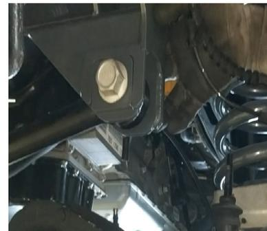
Reinstall the track bar into the Maxtrac track bar bracket using the OE bolt and adjustable cam plate. Torque to 406 ft. lbs.
