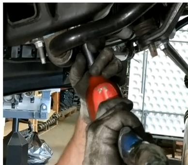
Unbolt the sway bar from the sway bar end links on both sides of the vehicle. Save the hardware for reuse.
