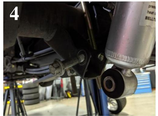
b) Remove the top shock bolt using a 15 mm wrench. The nut is flagged and will bind, allowing you to undo the bolt with no further tools. **(PHOTO 5)**
