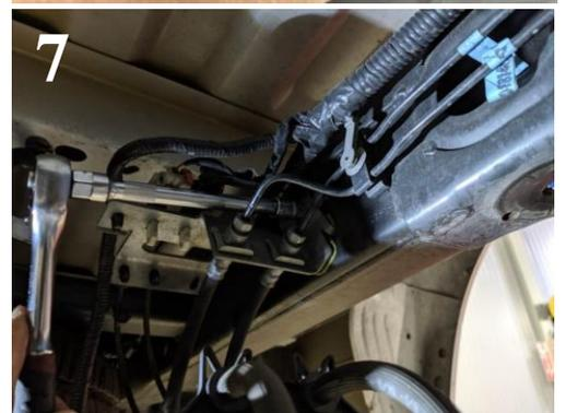
e) Using panel poppers, undo the wiring loom and brake lines from any surrounding mounting locations to allow for slack in the lines. **(PHOTO 8 & 9)**
