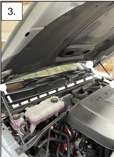
4. Attach the up-fitter harness to the 55" splitter harness. Route the clasp connectors on the upfitter harness to the relay box. Located on the driver side of the relay box are the upfitter wires. Pull the wires out and separate them.
