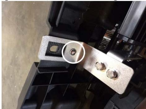
8. Now re-install the factory grille. Checking fitment. On certain year Super Duty's the horn sits lower than others. Slightly flex the bracket up and out of the way allowing for added clearance.
