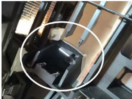
3. Remove the factory stud on the S8 light bar and install the supplied longer one.
