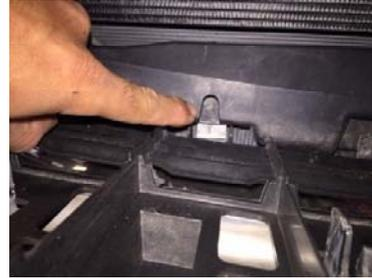
2. Use snips to cut the bridge part out of the grille as shown in the picture. You have the option of removing the entire plastic grille with snips for an un-obstructed view and for maximum performance of the light.
