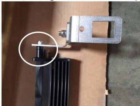
6. Now install the light and brackets onto the grille checking fitment. Tighten the 7/16 nut on the end of the light. It will not be accessible once installed.
