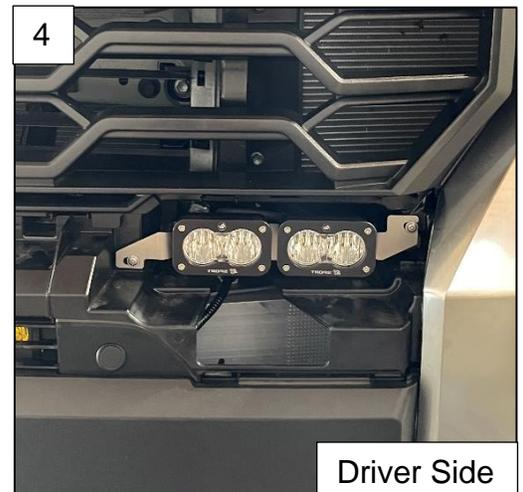
5. Repeat steps 2-4 for the passenger side. Check that the lights work when the vehicles fog lights are activated. Carefully reinstall the bumper cover starting near the grill bezels.
