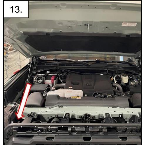
14. Run the switch lead along the firewall and to the wiring passthrough located to the right of the brake master cylinder.
