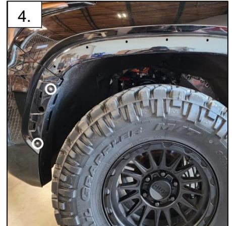
4. With a Phillips head screwdriver, remove the 2 silver screws (circled) attaching the front clip to the fender. Repeat step 3 and 4 for the passenger side of the vehicle.
