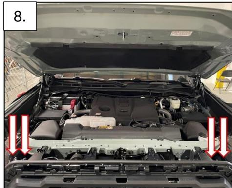
9. Using a trim tool or flathead screwdriver, remove the 2 plastic push rivets from either side of the grill near the previously disconnected electrical connectors.
