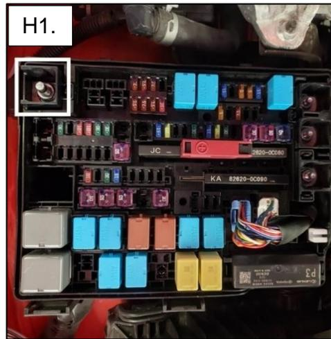
H2. Using a 12mm socket, remove the nut holding down the wire and release the tab to the right of the post. Lift to remove the wire and plastic wire cover.
