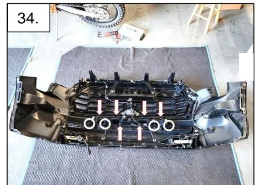
35. With a trim removal tool, carefully disengage the 27 tabs that hold the grill to the front clip. Remove the two reusable zip tie fasteners and TSS cover to use on the new grill.
