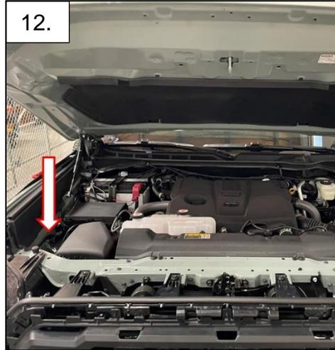
13. Locate the light connector lead of the wiring harness and starting at the battery, route it towards the radiator.
