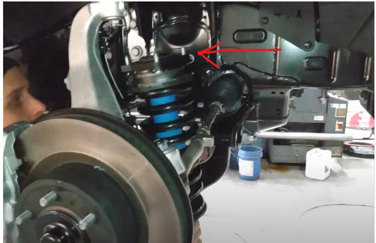
Install plates on top of strut
