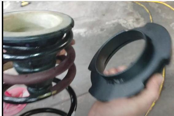
Put traxda spacer on top of spring isolator
