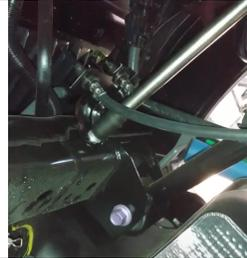
remove brackets for brake lines at differential
