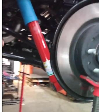
remove sway bar link at chassis
