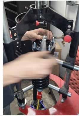
Install preload spacer, it will only fit one orientation.
