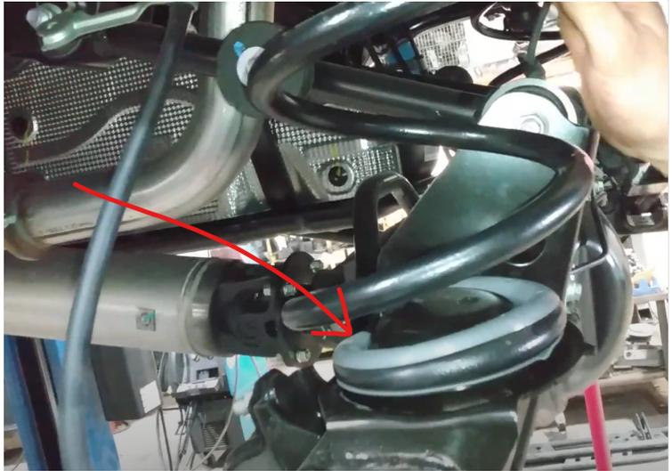
reinstall spring into truck, paying attention to pigtail on spring fits into pocket
