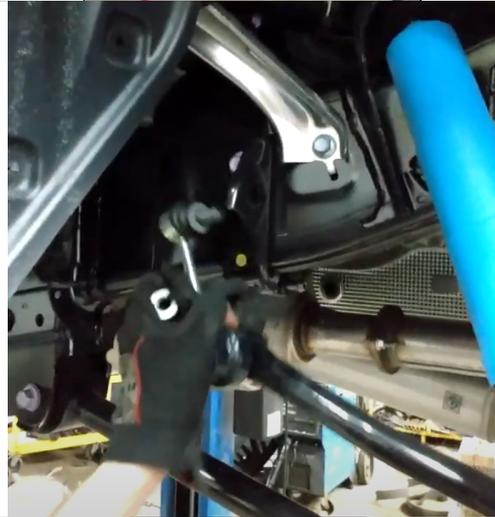
remove brackets holding brake lines on at chassis
