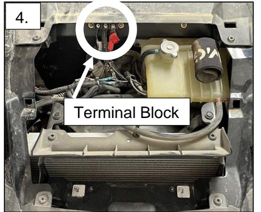
5. Using a 10mm socket, place the red ring terminal on the accessory post. Place the black terminal on the ground post. Route the switch through the firewall just below the terminal block.
