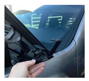
5. The bracket can now be moved into position carefully as to not scratch the body of the vehicle.
