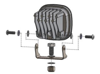
10. Now with the 9/16" wrench and socket, the lights can be placed onto the A-pillar brackets, aimed, and tightened.
