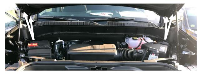
2. Place masking tape along the hood hinges (shown below) to ensure proper alignment.
